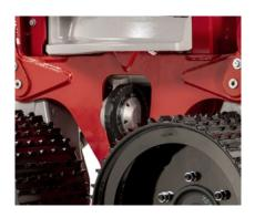
Updated attachment for the expander pin to measuring wheel arm to simplifying service and maintenance.
