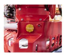
In order to facilitate maintenance work, 6000V has easy access lubrication points. All lubrication can be done when the unit is in raised position which increases safety and shortens downtime.
