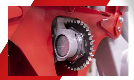
To offer the best measurement results, we've made some changes in the length measurement function. We have updated the construction of the measure wheel cylinder, the hydraulic circuit and reinforced the measuring wheel arm and its attachment. We also have a completely new measuring wheel unit including a bigger measuring wheel. Altogether, the changes will allow the measuring wheel to follow the contour of the stem even better and provide the best measurement result.
