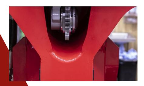
To improve the frame's durability and life span, we have changed the design of the measuring wheel hole. We also reinforced the stoppers for the roller arms, when in closed position, at the inside of the frame to increase the frame's strength and stability.
